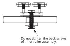
The roller assembly must be loosely fixed on glass at this time.
