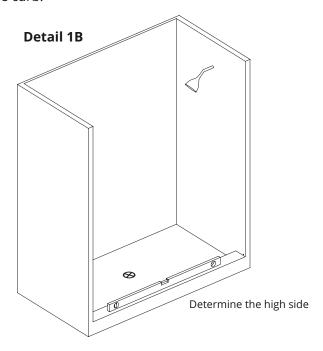
**STEP 2 Use a level to** determine the exact vertical plumb position of the pencil line that extends the centerline on the vertical wall.
