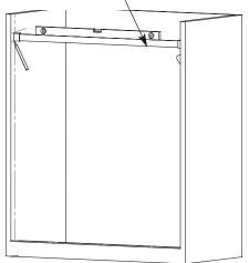
**Detail 5C**Drill the holes and fasten the second Header Bracket to the wall.
