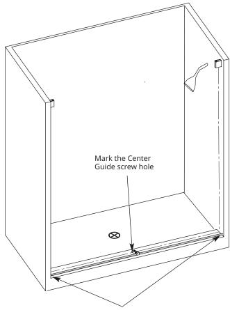
Mark the position of the Curb Dam with pencil lines at each end on the wall and across the outside edge of the Curb Dam on the base.
