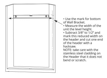
**STEP 3. Drill and install the install the Header Wall Bracket** Use the Flathead Screws and anchors as supplied.
