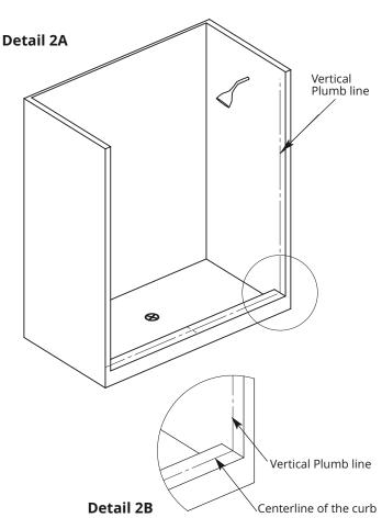
**STEP 2C**. Using the penciled centerline on the wall use a level to recheck the exact vertical position. Mark the top height for the unit at 66" or 76".
