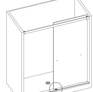
Position the Curb Dam pencil mark for outside edge 1 15/32" from the center line.
