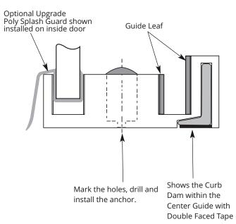
**STEP 14**. Turn the Curb Dam over. Remove the film covering the double faced tape. Carefully align one end of the Curb Dam to the pencil marks on the wall and lower it into place to align with the pencil marks on the curb. Fit the Center Guide into place over the screw hole by sliding it over the Curb Dam and under the Inside Door.
