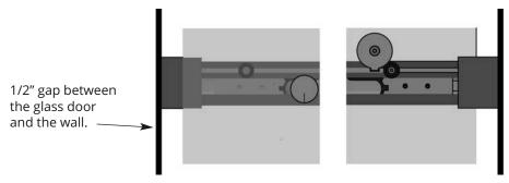
Tighten both Inner and Outer Door Stops on both doors at this position at the ends of the Header in to prevent the glass doors from hitting the wall.
