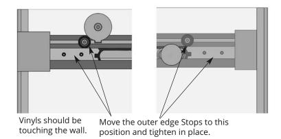
Detail 18B -- Shows Doors fully open with 1/2" gap to the wall
